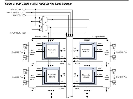
Figure 2 shows the architecture of MAX 7000E and MAX 7000S devices.
