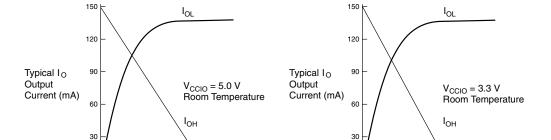
Figure 11. Output Drive Characteristics of 5.0-V MAX 7000 Devices
