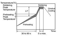
[Allowable Flow Soldering Temperature and Time]
