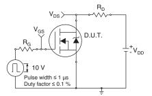
Fig. 10a - Switching Time Test Circuit
