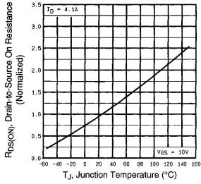
Fig. 4 - Normalized On-Resistance vs. Temperature
