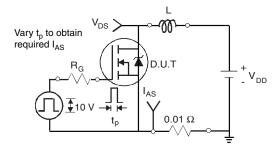
Fig. 12a - Unclamped Inductive Test Circuit
