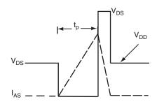
Fig. 12b - Unclamped Inductive Waveforms
