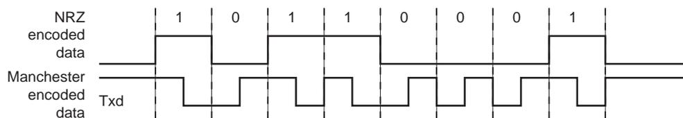
The Manchester encoded character can also be encapsulated by adding both a configurable preamble and a start frame delimiter pattern. Depending on the configuration, the preamble is a training sequence, composed of a
