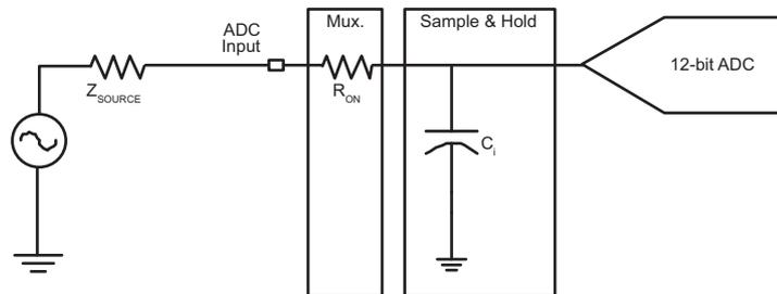
In 12-bit mode, during the tracking phase, the ADC needs to track the input signal during the tracking time shown below:
