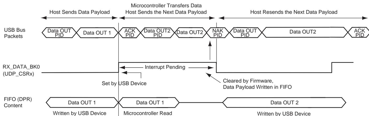
An interrupt is pending while the flag `RX_DATA_BK0` is set. Memory transfer between the USB device, the FIFO and microcontroller memory is not possible after `RX_DATA_BK0` has been cleared. Otherwise, the USB device would accept the next Data OUT transfer and overwrite the current Data OUT packet in the FIFO.
