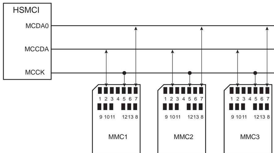
Note: When several HSMCI (x HSMCI) are embedded in a product, MCCK refers to HSMCIx\_CK, MCCDA to HSMCIx\_CDA, MCDy to HSMCIx\_Dy.
