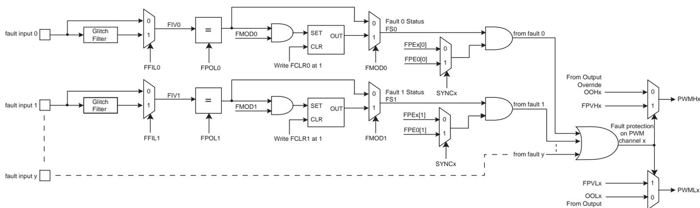
The polarity level of the fault inputs is configured by the FPOL field in the [PWM Fault Mode Register \(PWM\\_FMR\)](#). For fault inputs coming from internal peripherals such as ADC or Timer Counter, the polarity level must be FPOL = 1. For fault inputs coming from external GPIO pins the polarity level depends on the user's implementation.
