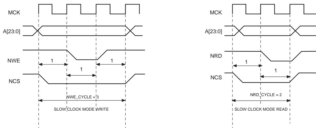
Table 26-6. Read and Write Timing Parameters in Slow Clock Mode
