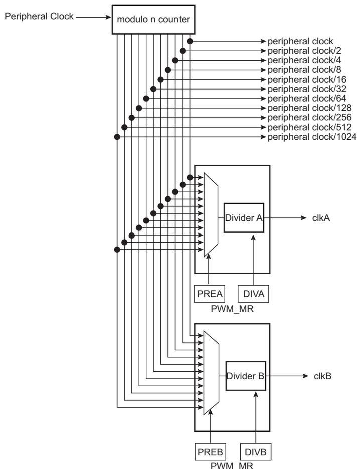
The PWM peripheral clock is divided in the clock generator module to provide different clocks available for all channels. Each channel can independently select one of the divided clocks.
