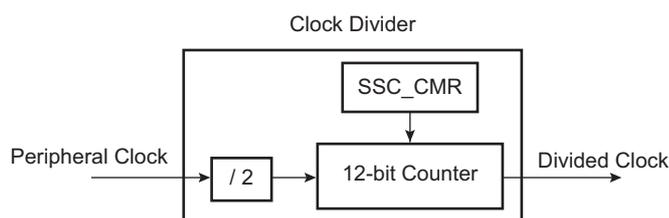
The peripheral clock divider is determined by the 12-bit field DIV counter and comparator (so its maximal value is 4095) in the Clock Mode Register (SSC\_CMCR), allowing a peripheral clock division by up to 8190. The Divided Clock is provided to both the Receiver and Transmitter. When this field is programmed to 0, the Clock Divider is not used and remains inactive.
