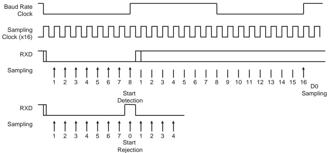
**Figure 36-12. Asynchronous Character Reception**
