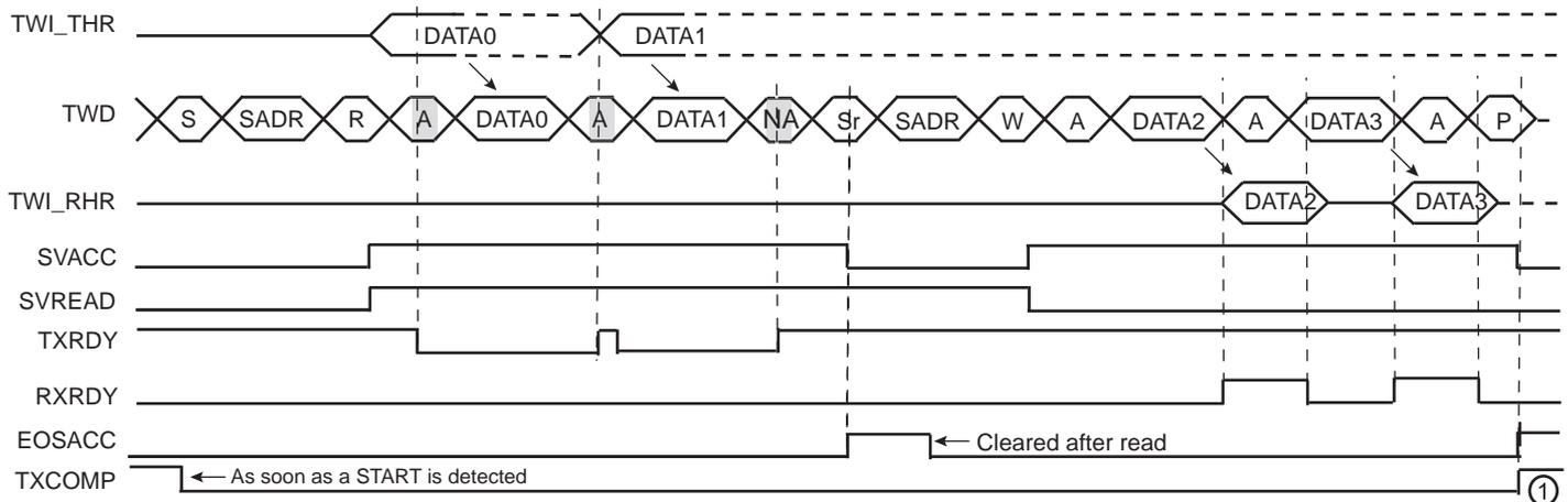
Note: 1. TXCOMP is only set at the end of the transmission because after the repeated start, SADR is detected again.
