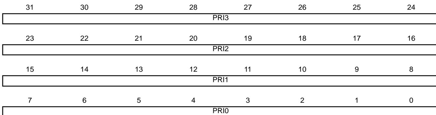
The NVIC\_IPR0–NVIC\_IPR8 registers provide a 8-bit priority field for each interrupt. These registers are byte-accessible. Each register holds four priority fields that map up to four elements in the CMSIS interrupt priority array IP[0] to IP[34].
