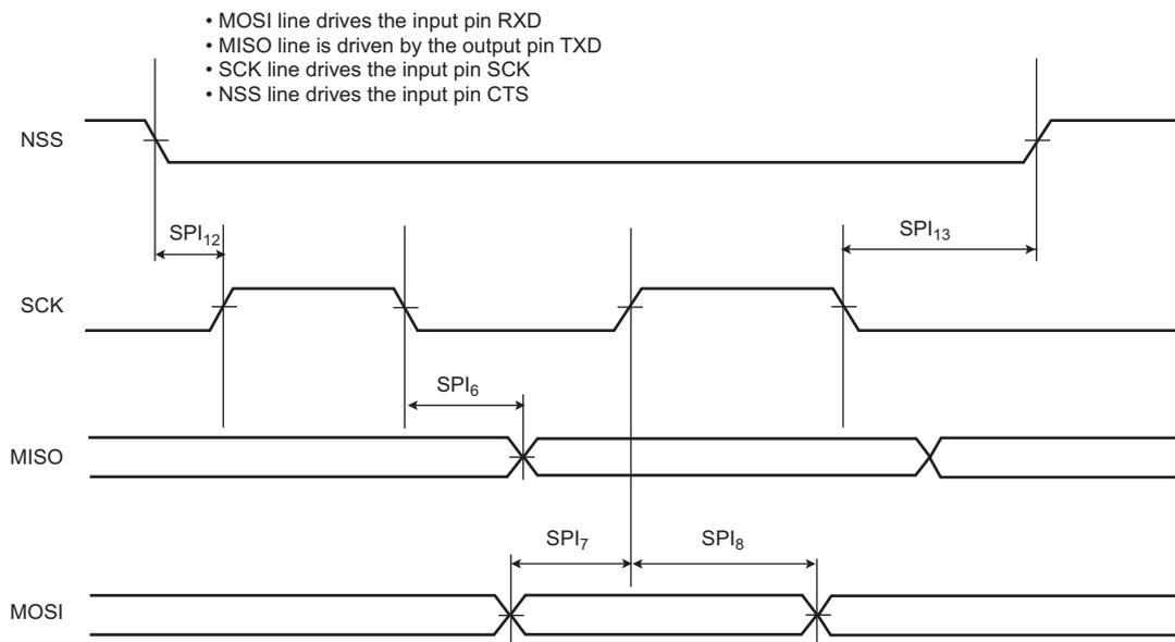
Figure 44-39. USART SPI Slave Mode: (Mode 0 or 3)
