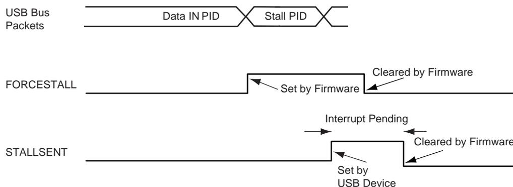
**Figure 40-13. Stall Handshake (Data OUT Transfer)**
