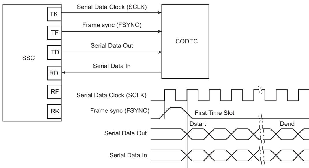
**Figure 32-5. Time Slot Application Block Diagram**
