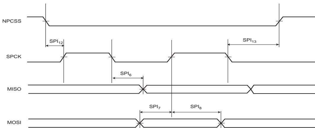
**Figure 44-25. SPI Slave Mode with (CPOL = NCPHA = 0) or (CPOL = NCPHA = 1)**
