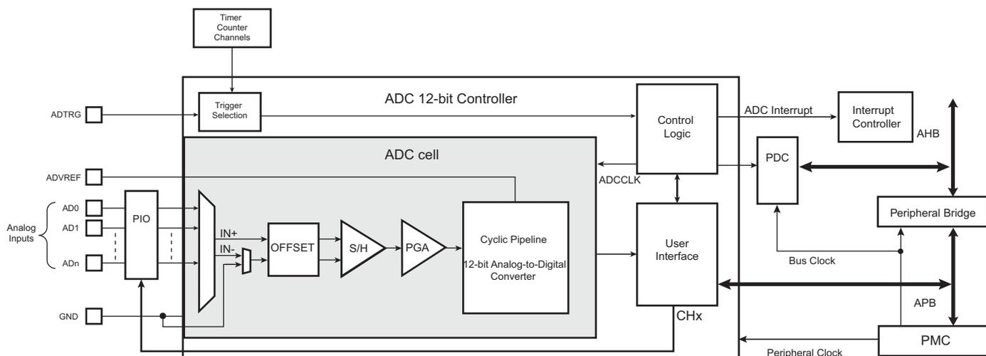
Note: DMA may be referred to as PDC (Peripheral DMA Controller).
