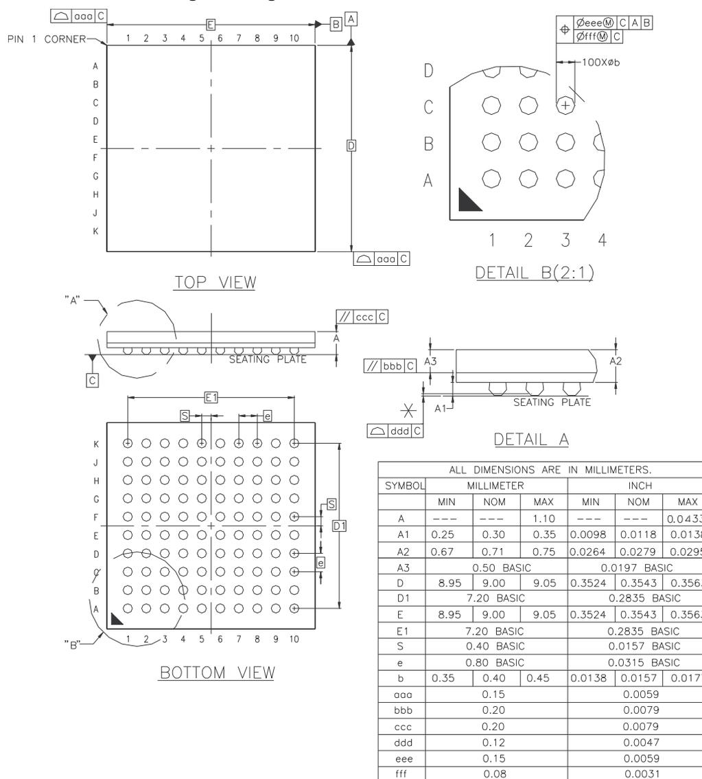
Table 45-4. TFBGA Package Reference - Soldering Information (Substrate Level)
