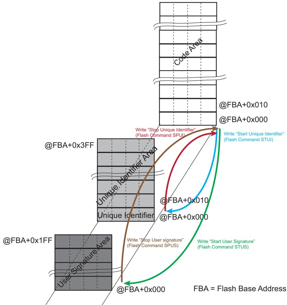
Figure 20-2. Organization of Embedded Flash for Code
