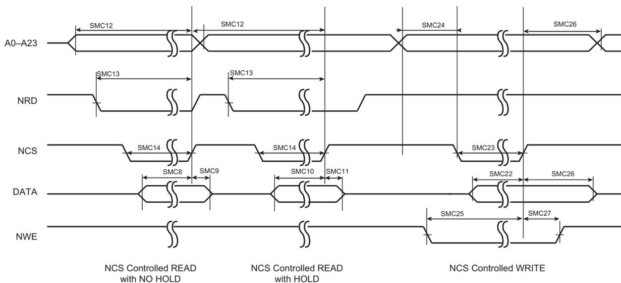
**Figure 44-36. SMC Timings - NRD Controlled Read and NWE Controlled Write**
