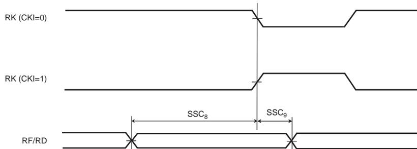
**Figure 44-31. SSC Receiver, RK as Input and RF as Output**
