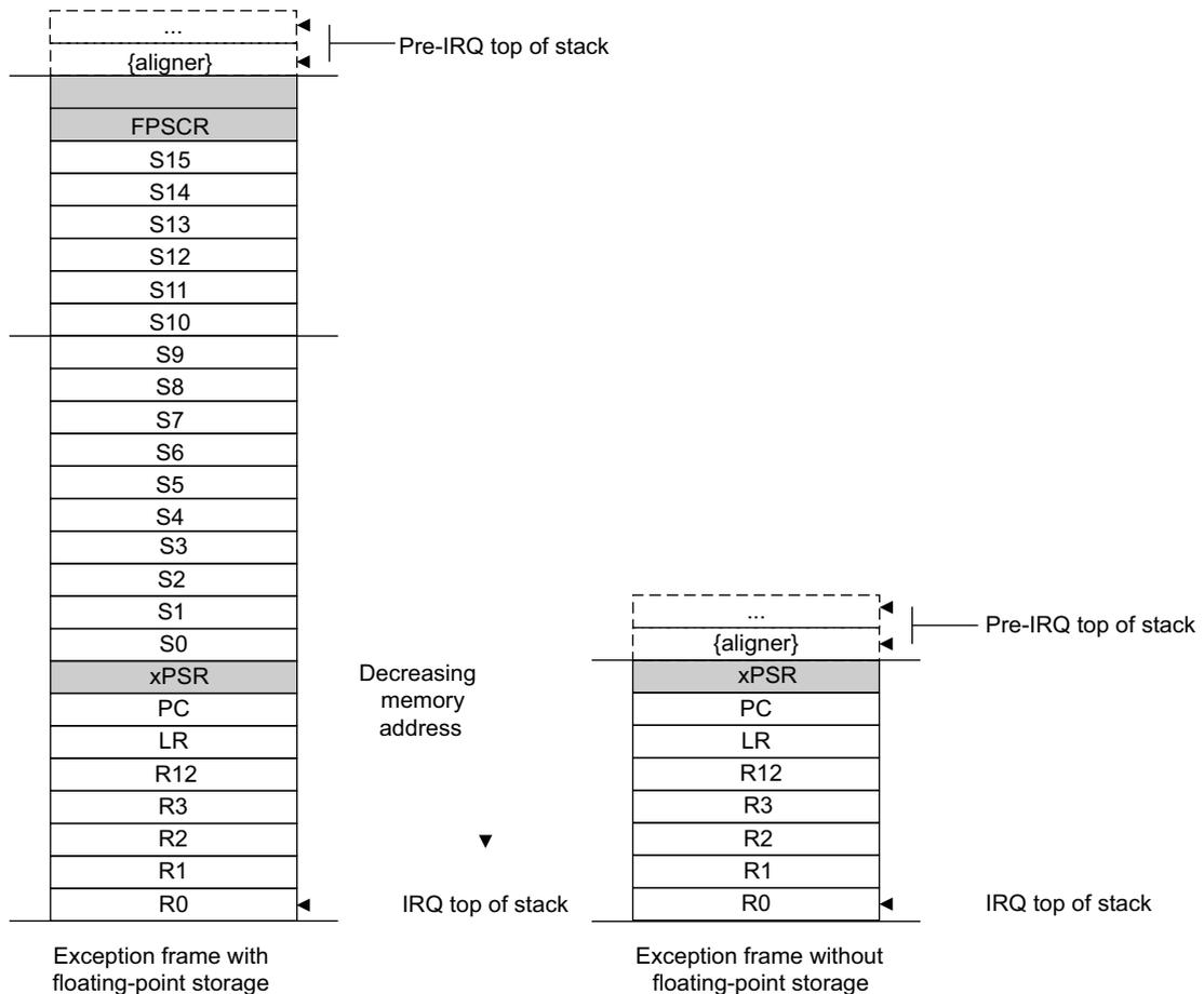
Immediately after stacking, the stack pointer indicates the lowest address in the stack frame. The alignment of the stack frame is controlled via the STKALIGN bit of the Configuration Control Register (CCR).
