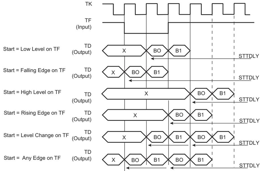
**Figure 32-14. Receive Pulse/Edge Start Modes**
