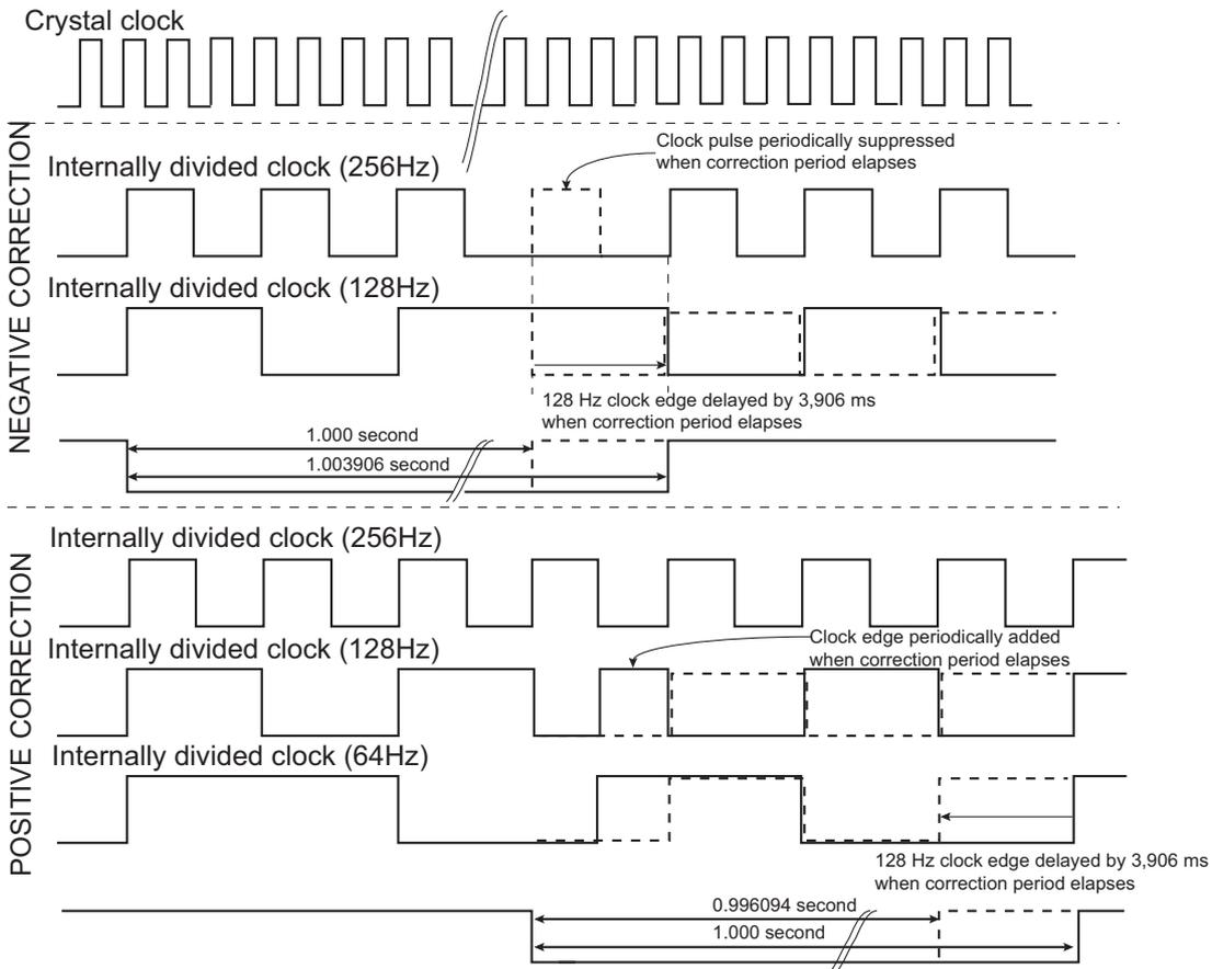
The inaccuracy of a crystal oscillator at typical room temperature ( $\pm 20$  ppm at 20–25 °C) can be compensated if a reference clock/signal is used to measure such inaccuracy. This kind of calibration operation can be set up during
