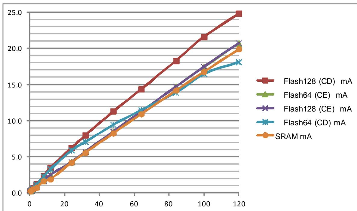
**Table 44-24. SAM4SD32/SA16/SD16 Typical Active Power Consumption with VDDCORE@ 1.2V running from Flash Memory (AMP2) or SRAM**
