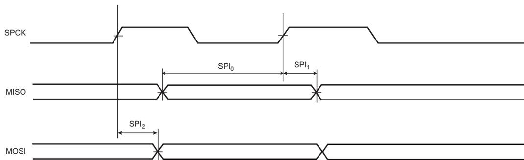
**Figure 44-23. SPI Master Mode with (CPOL = 0 and NCPHA = 1) or (CPOL = 1 and NCPHA = 0)**
