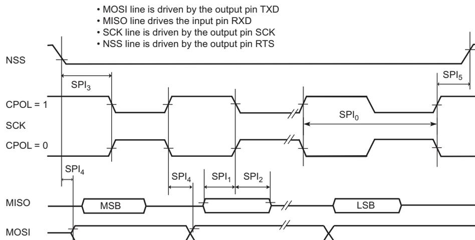
**Figure 44-38. USART SPI Slave Mode: (Mode 1 or 2)**
