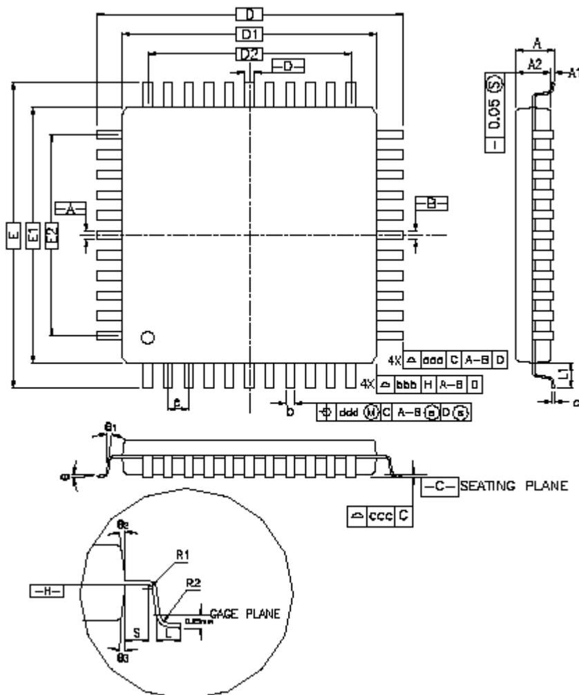
Table 45-13. 64-lead LQFP Package Dimensions (in mm)
