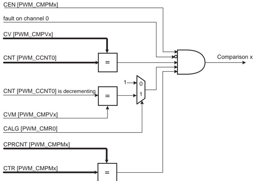
The comparison x matches when it is enabled by the bit CEN in the [PWM Comparison x Mode Register](#) (PWM\_CMPMx for the comparison x) and when the counter of the channel 0 reaches the comparison value defined by the field CV in [PWM Comparison x Value Register](#) (PWM\_CMPVx for the comparison x). If the counter
