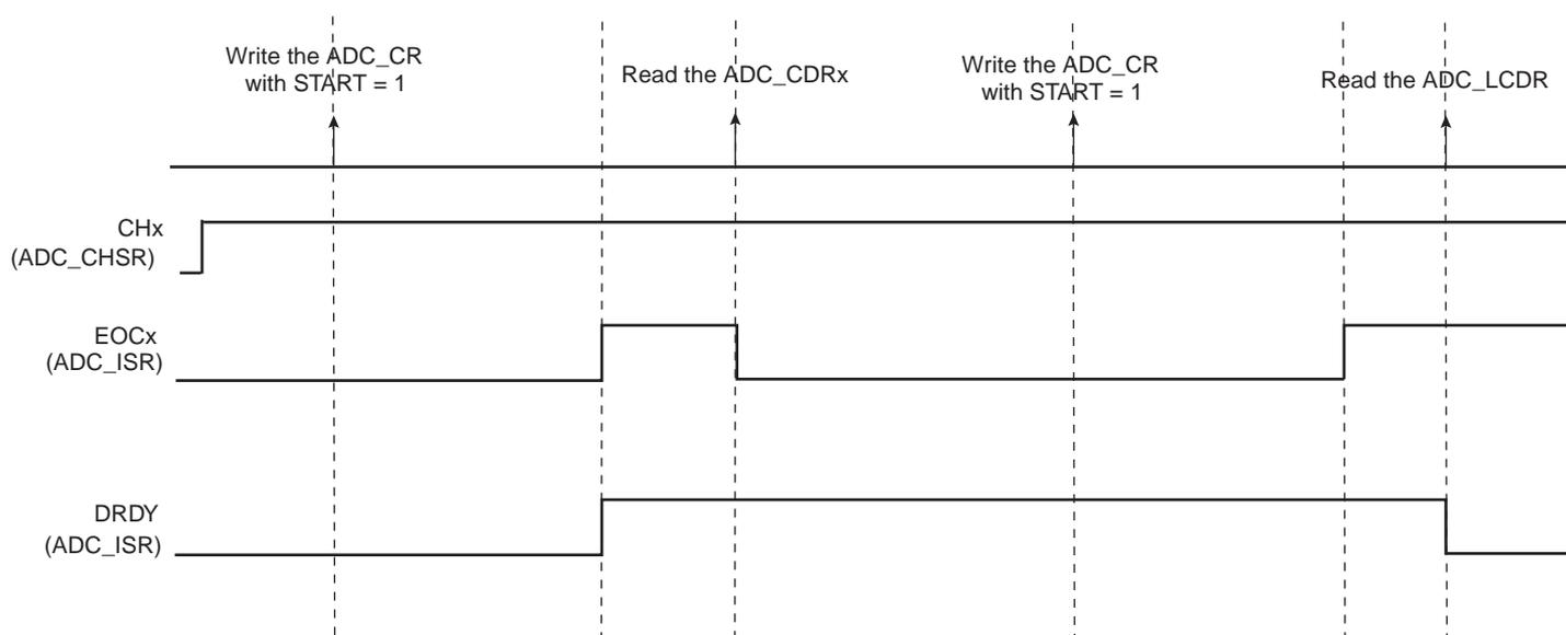
If ADC\_CDR is not read before further incoming data is converted, the corresponding OVREx flag is set in the Overrun Status register (ADC\_OVER).
