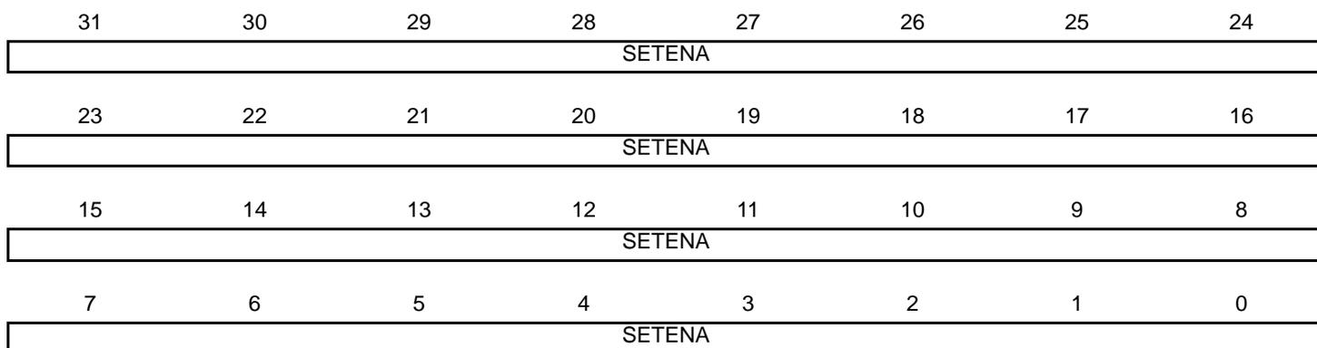
These registers enable interrupts and show which interrupts are enabled.
