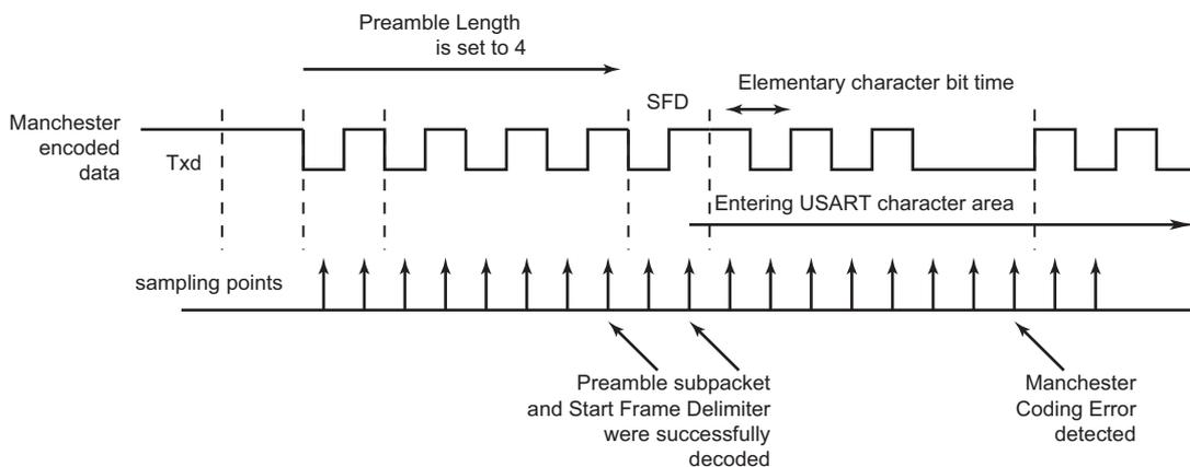
When the start frame delimiter is a sync pattern (ONEBIT field to 0), both command and data delimiter are supported. If a valid sync is detected, the received character is written as RXCHR field in the US\_RHR and the RXSYNH is updated. RXCHR is set to 1 when the received character is a command, and it is set to 0 if the received character is a data. This mechanism alleviates and simplifies the direct memory access as the character contains its own sync field in the same register.
