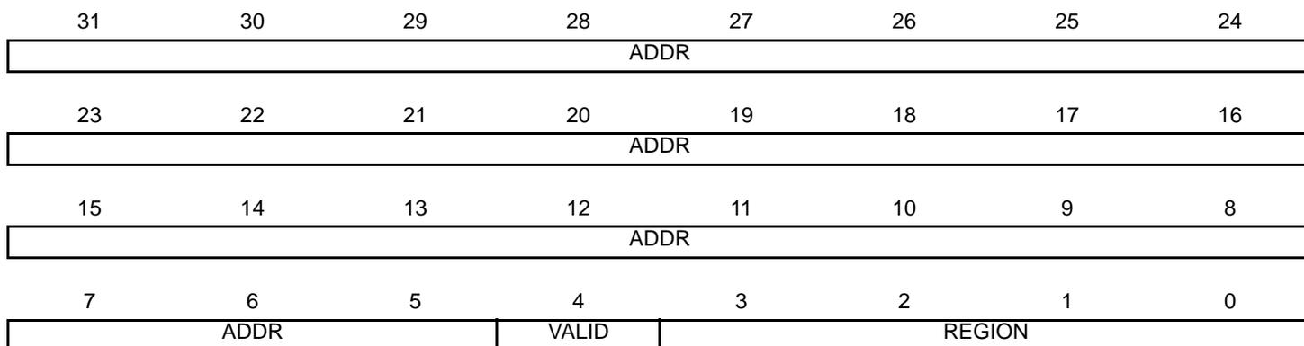
The MPU\_RBAR defines the base address of the MPU region selected by the MPU\_RNR, and can update the value of the MPU\_RNR.
