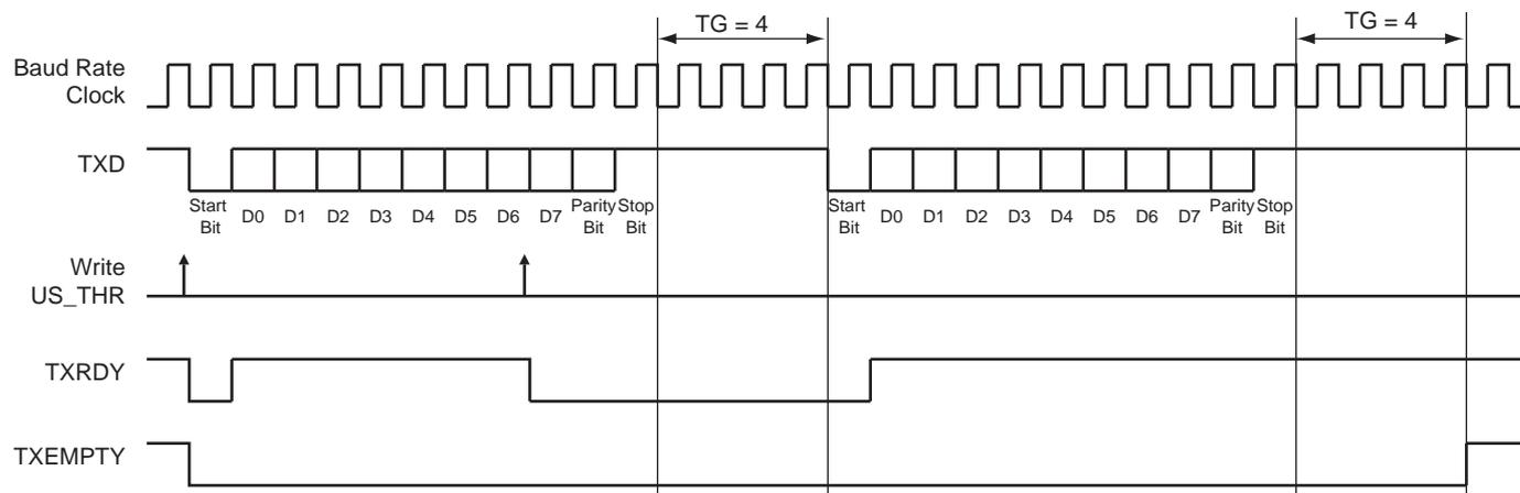
Table 36-9 indicates the maximum length of a timeguard period that the transmitter can handle in relation to the function of the baud rate.
