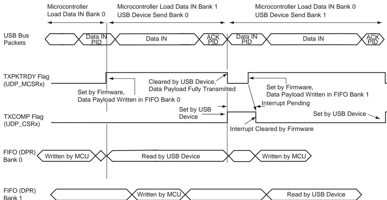
**Warning:** There is software critical path due to the fact that once the second bank is filled, the driver has to wait for TX\_COMP to set TX\_PKTRDY. If the delay between receiving TX\_COMP is set and TX\_PKTRDY is set too long, some Data IN packets may be NACKed, reducing the bandwidth.
