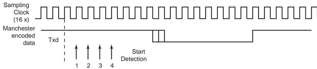
The receiver is activated and starts preamble and frame delimiter detection, sampling the data at one quarter and then three quarters. If a valid preamble pattern or start frame delimiter is detected, the receiver continues decoding with the same synchronization. If the stream does not match a valid pattern or a valid start frame delimiter, the receiver resynchronizes on the next valid edge. The minimum time threshold to estimate the bit value is three quarters of a bit time.
