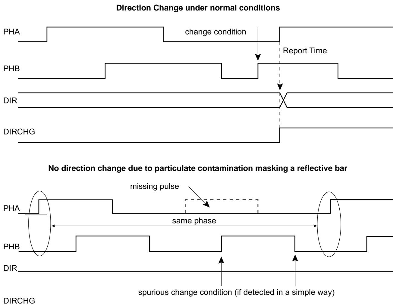
The direction change detection is disabled when QDTRANS is set in the TC\_BMR. In this case, the DIR flag report must not be used.
