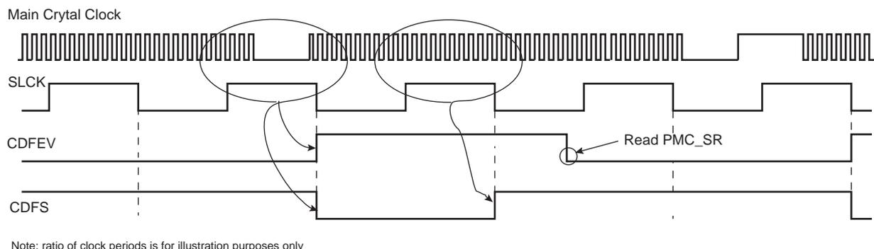
If the main oscillator is selected as the source clock of MAINCK (MOSCSEL in CKGR\_MOR = 1), and if the master clock source is PLLACK or PLLBCK (CSS = 2 or 3), a clock failure detection automatically forces MAINCK to be the source clock for the master clock (MCK). Then, regardless of the PMC configuration, a clock failure detection
