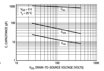
Figure 7b. High Voltage Capacitance Variation
