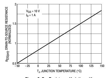
Figure 5. On-Resistance Variation with Temperature
