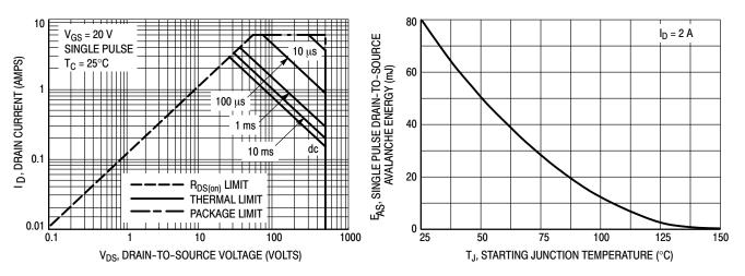
Figure 11. Maximum Rated Forward Biased Safe Operating Area
