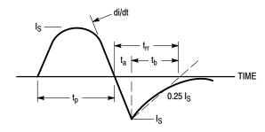
Figure 14. Diode Reverse Recovery Waveform
