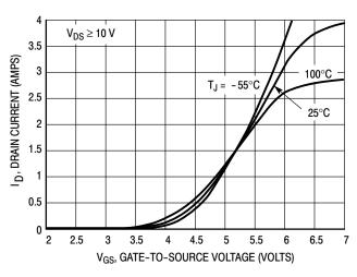
Figure 2. Transfer Characteristics
