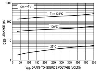
Figure 6. Drain-To-Source Leakage Current versus Voltage
