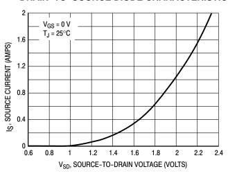
Figure 10. Diode Forward Voltage versus Current
