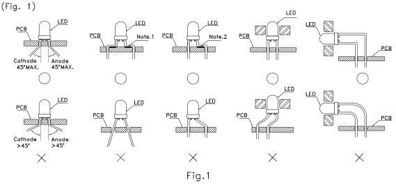
" $\bigcirc$ " Correct mounting method " $\times$ " Incorrect mounting method Note 1-2: Do not route PCB trace in the contact area between the leadframe and the PCB to prevent short-circuits.
