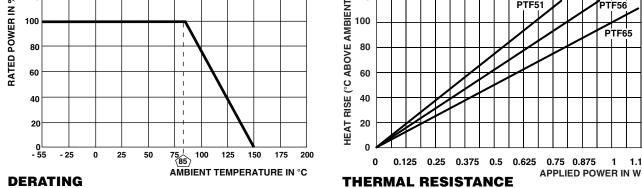
Example: When a PTF56 part is run at 1/8 W in a 70 °C ambient environment, the resistor will generate enough heat that the surface temperature of the part will reach about 17 °C over the ambient temperature, and over the life of the part this could cause the resistance value to shift up to  $\pm 0.04$  %.
