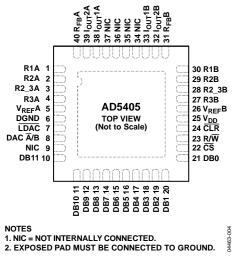
Figure 4. Pin Configuration
