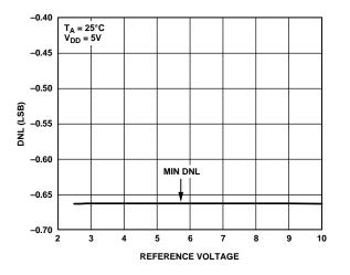
Figure 8. Differential Nonlinearity (DNL) vs. Reference Voltage
