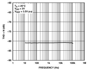
Figure 20. THD and Noise vs. Frequency
