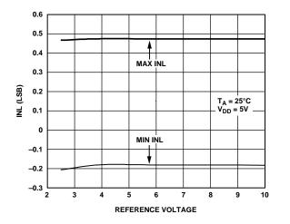
Figure 7. INL vs. Reference Voltage
