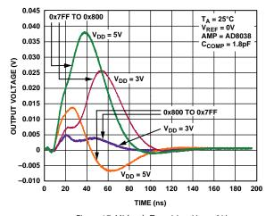
Figure 17. Midscale Transition,  $V_{REF} = 0 V$
