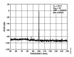
Figure 27. Narrow-Band SFDR,  $f_{OUT} = 100 \text{ kHz}$ , Clock = 25 MHz
