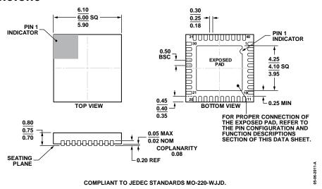
Figure 44. 40-Lead Lead Frame Chip Scale Package [LFCSP] 6 mm × 6 mm Body and 0.75 mm Package Height (CP-40-9) Dimensions shown in millimeters
