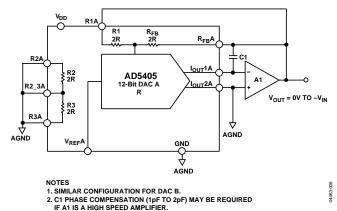
Figure 32. Unipolar Operation
