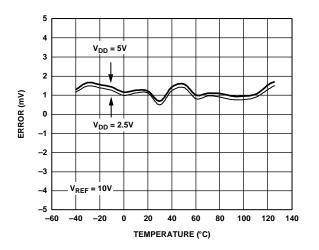
Figure 9. Gain Error vs. Temperature
