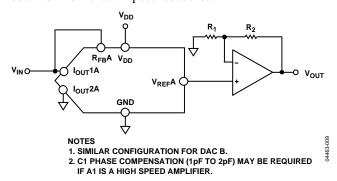
Figure 34. Single-Supply Voltage-Switching Mode
