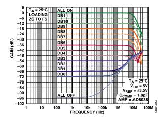
Figure 14. Reference Multiplying Bandwidth vs. Frequency and Code
