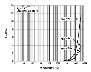
Figure 13. Supply Current vs. Update Rate
