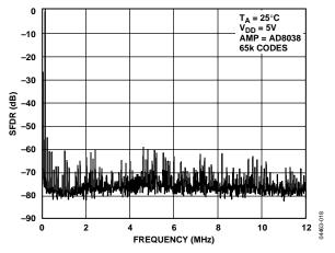
Figure 23. Wideband SFDR,  $f_{OUT} = 100 \text{ kHz}$ , Clock = 25 MHz
