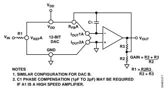
Figure 35. Increasing Gain of Current Output DAC
