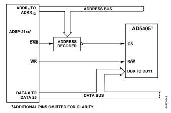
Figure 37. ADSP-21xx to AD5405 Interface
