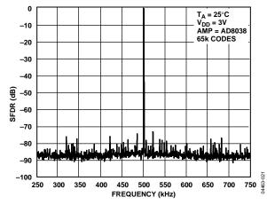
Figure 26. Narrow-Band Spectral Response,  $f_{OUT} = 500 \text{ kHz}$ , Clock = 25 MHz
