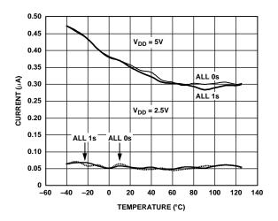
Figure 12. Supply Current vs. Temperature
