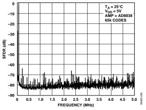
Figure 25. Wideband SFDR,  $f_{OUT} = 50 \text{ kHz}$ , Clock = 10 MHz
