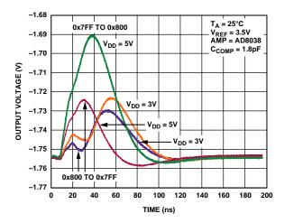
Figure 18. Midscale Transition,  $V_{REF} = 3.5 V$
