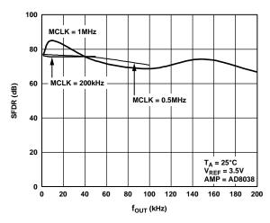
Figure 21. Wideband SFDR vs. fout Frequency
