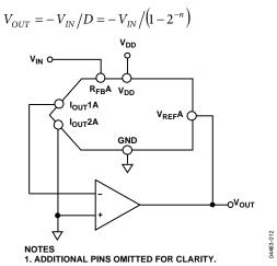
Figure 36. Current Steering DAC Used as a Divider or Programmable Gain Element
