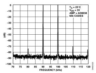
Figure 28. Narrow-Band IMD,  $f_{OUT} = 90 \text{ kHz}$ , 100 kHz, Clock = 10 MHz
