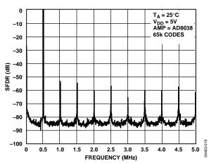
Figure 24. Wideband SFDR,  $f_{OUT} = 500 \text{ kHz}$ , Clock = 10 MHz
