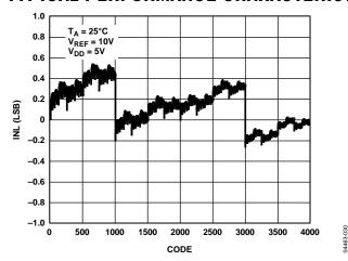
Figure 5. Integral Nonlinearity (INL) vs. Code (12-Bit DAC)
