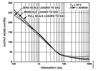
Figure 30. Output Noise Spectral Density
