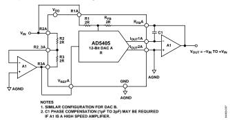
Figure 33. Bipolar Operation (4-Quadrant Multiplication)
