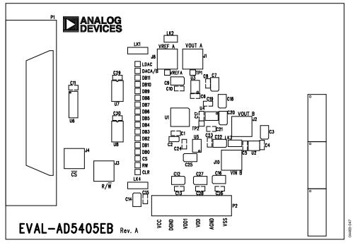
Figure 42. Silkscreen—Component Side View (Top Layer)
