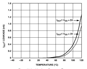
Figure 11. IOUT1 Leakage Current vs. Temperature
