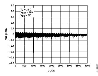
Figure 6. DNL vs. Code (12-Bit DAC)
