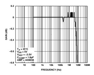
Figure 15. Reference Multiplying Bandwidth—All 1s Loaded
