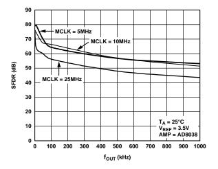
Figure 22. Wideband SFDR vs. f<sub>OUT</sub> Frequency
