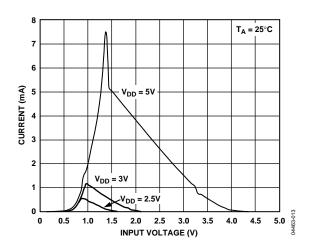
Figure 10. Supply Current vs. Logic Input Voltage
