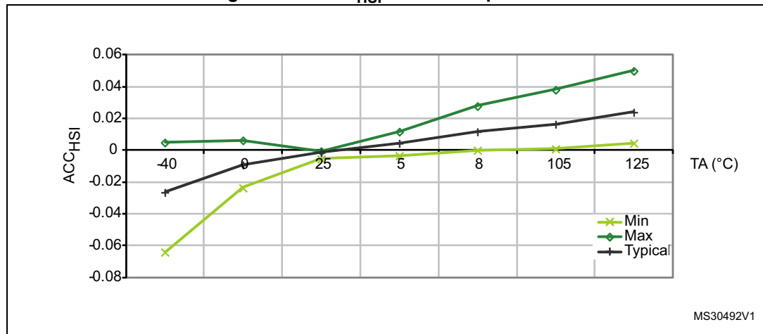
Figure 27. LACC_{HSI} versus temperature
