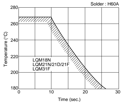
Allowable Flow Soldering Temperature and Time
