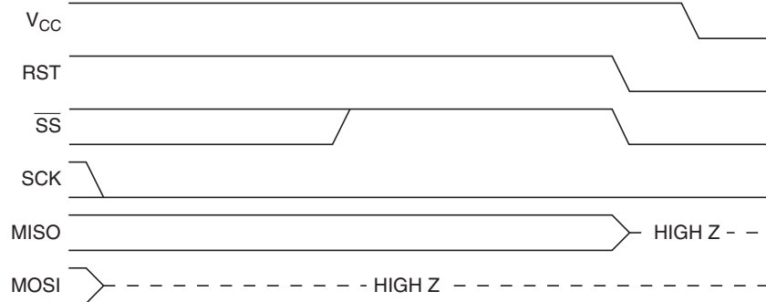
Figure 23-23. Serial Programming Power-down Sequence
