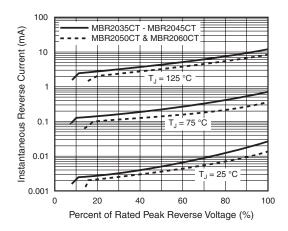
Figure 4. Typical Reverse Characteristics Per Diode
