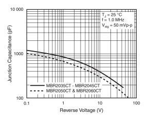
Figure 5. Typical Junction Capacitance Per Diode
