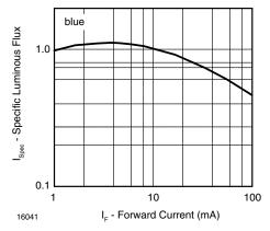
Fig. 6 - Specific Luminous Flux vs. Forward Current
