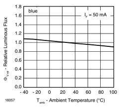
Fig. 7 - Rel. Luminous Flux vs. Ambient Temperature
