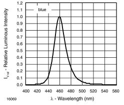
Fig. 3 - Relative Intensity vs. Wavelength
