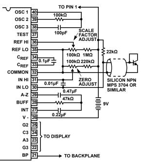
A silicon diode-connected transistor has a temperature coefficient of about -2mV/°C. Calibration is achieved by placing the sensing transistor in ice water and adjusting the zeroing potentiometer for a 000.0 reading. The sensor should then be placed in boiling water and the scale-factor potentiometer adjusted for a 100.0 reading.
