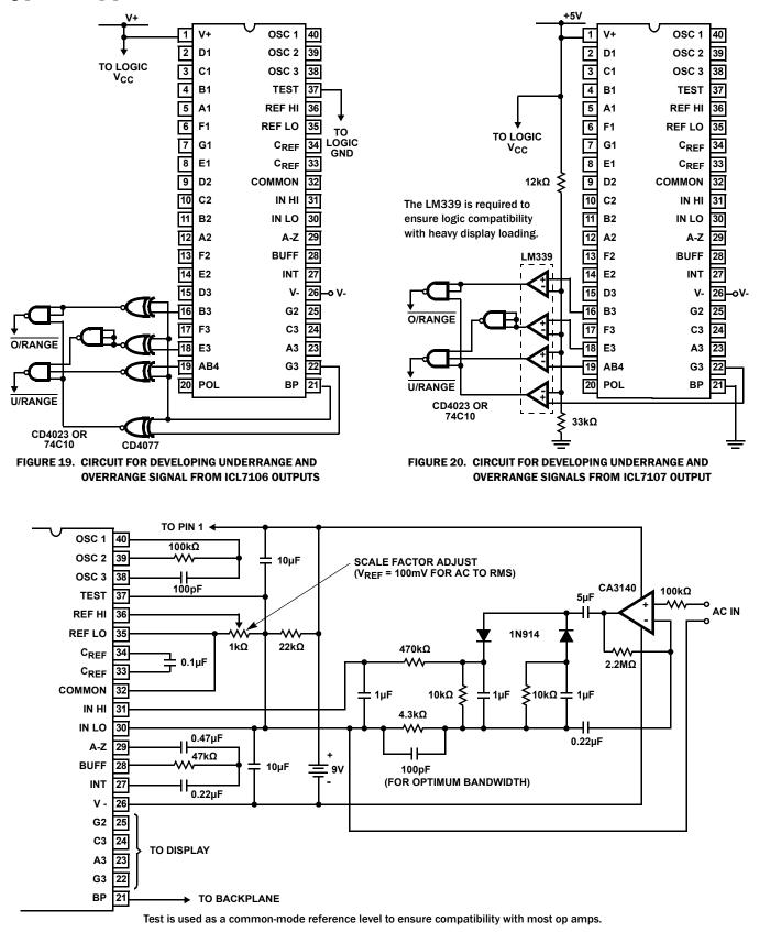
FIGURE 21. AC TO DC CONVERTER WITH ICL7106
