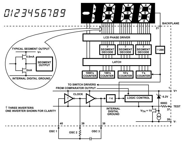
FIGURE 7. ICL7106 DIGITAL SECTION
