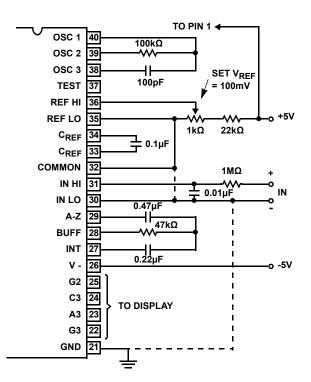
Values shown are for 200mV full scale, 3 readings/sec. IN LO may be tied to either COMMON for inputs floating with respect to supplies, or GND for single ended inputs. (See discussion in <u>"Analog COMMON" on page 7.</u>)
