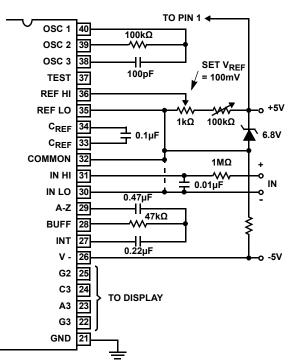
Since low TC zeners have breakdown voltages ~ 6.8V, diode must be placed across the total supply (10V). As in the case of <u>Figure 12</u>, IN LO may be tied to either COMMON or GND.
