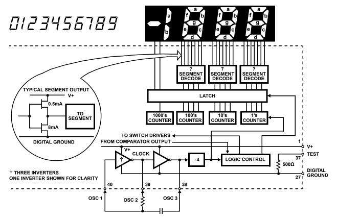
FIGURE 8. ICL7107 DIGITAL SECTION
