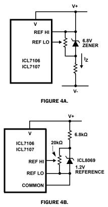
FIGURE 4. USING AN EXTERNAL REFERENCE
