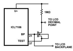
FIGURE 5. SIMPLE INVERTER FOR FIXED DECIMAL POINT
