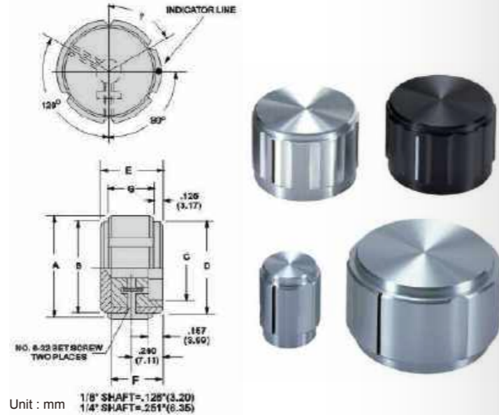
Unit : mm 1/8" SHAFT=.126*(3.20) 1/4" SHAFT=.251*(6.35)
