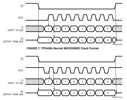
FIGURE 8. TP3420A Alternate MICROWIRE Clock Format
