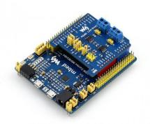
RS485 CAN Shield Designed for NUCLEO/XNUCLEO
