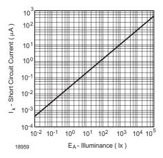
Figure 3. Short Circuit Current vs. Illuminance
