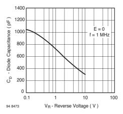
Figure 6. Diode Capacitance vs. Reverse Voltage
