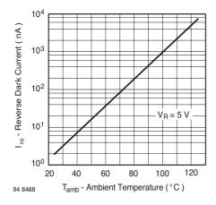
Figure 1. Reverse Dark Current vs. Ambient Temperature
