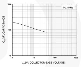
**Figure 4. Collector Output Capacitance**
