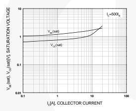
Figure 3. Collector-Emitter Saturation Voltage and Base-Emitter Saturation Voltage
