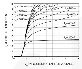
Figure 1. Static Characteristic
