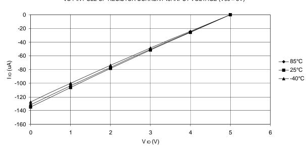
VO PIN PULL-UP RESISTOR CURRENT vs. INPUT VOLTAGE (Vcc = 5V)
