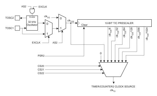
The clock source for Timer/Counter2 is named  $clk_{T2S}$ .  $clk_{T2S}$  is by default connected to the main system I/O clock  $clk_{IO}$ . By setting the AS2 bit in ASSR, Timer/Counter2 is asynchronously clocked from the TOSC oscillator or TOSC1 pin. This enables use of Timer/Counter2 as a Real Time Counter (RTC).
