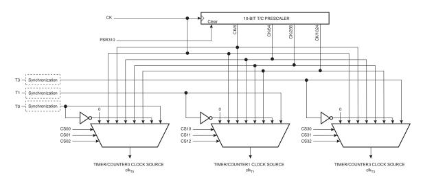
Note: 1. The synchronization logic on the input pins (T0/T1/T3) is shown in Figure 11-1.
