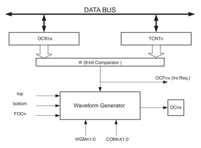
The OCR0A Register is double buffered when using any of the Pulse Width Modulation (PWM) modes. For the normal and Clear Timer on Compare (CTC) modes of operation, the double buffering is disabled. The double buffering synchronizes the update of the OCR0A Compare Register to either top or bottom of the counting sequence. The synchronization prevents the occurrence of odd-length, non-symmetrical PWM pulses, thereby making the output glitch-free.
