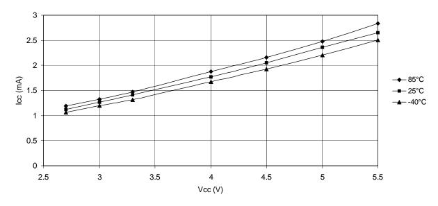
Figure 28-5. Active Supply Current vs. Vcc (32 kHz Watch Crystal)
