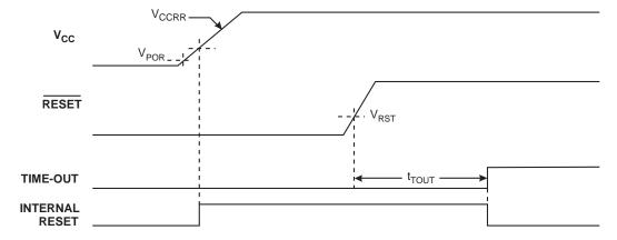
Note: If  $V_{POR}$  or  $V_{CCRR}$  parameter range can not be followed, an External Reset is required.
