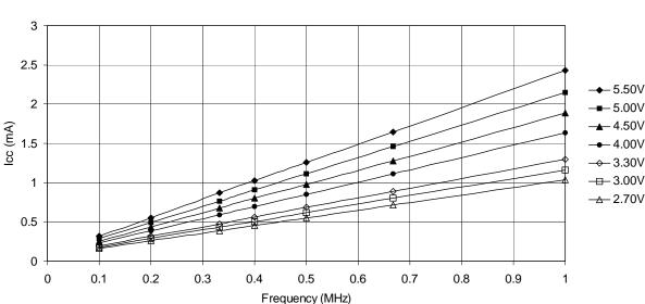
ACTIVE SUPPLY CURRENT vs. FREQUENCY (25°C, 0.1 - 1 MHz)
