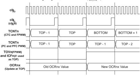
Figure 13-13. Timer/Counter Timing Diagram, with Prescaler ( $f_{clk}$   $_{I/O}$ /8)
