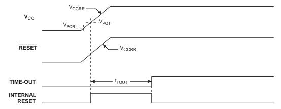
Figure 7-3. MCU Start-up, RESET Extended Externally
