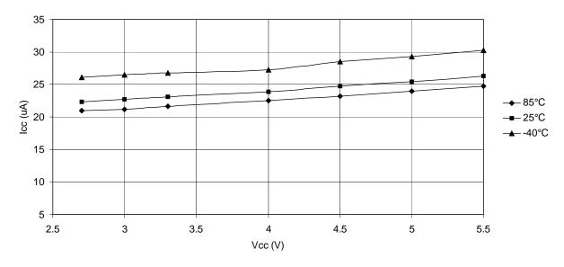
Figure 28-33. ADC Current vs. Operating Voltage (ADC at 1 MHz)
