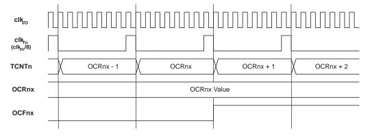
Figure 14-12 shows the setting of OCF2A and the clearing of TCNT2 in CTC mode.
