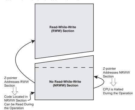
Figure 24-1. Read-While-Write vs. No Read-While-Write
