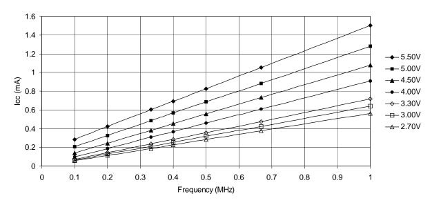
Figure 28-7. Idle Supply Current vs. Frequency (1 - 16 MHz)
