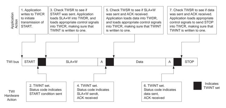
1. The first step in a TWI transmission is to transmit a START condition. This is done by writing a specific value into TWCR, instructing the TWI hardware to transmit a START condition. Which value to write is described later on. However, it is important that the TWINT bit is set in the value written. Writing a one to TWINT clears the flag. The TWI will not start any operation as long as the TWINT bit in TWCR is set. Immediately after
