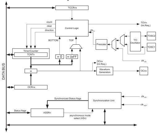
Figure 14-1. 8-bit Timer/Counter2 Block Diagram
