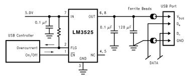
Figure 3. Typical Application Circuit
