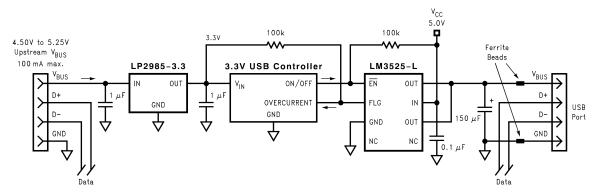
Figure 16. Single-Port USB Self-Powered Hub
