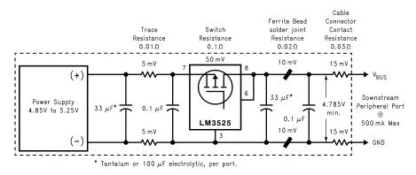
Figure 15. Self-Powered Hub Per-Port Voltage Drop
