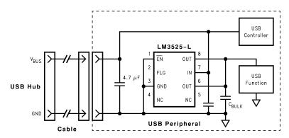
Figure 18. Inrush Current-limit Application
