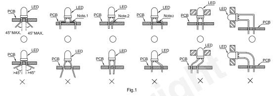
$\bigcirc$ " Correct mounting method "imes" Incorrect mounting method
